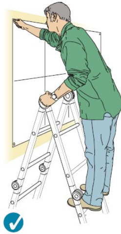
Figure 11 Correct - two clear rungs. Don't work any higher up this type of stepladder
