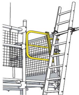
Figure 8 Access ladders should be tied and extend at least 1 m above the landing point to provide a secure handhold
