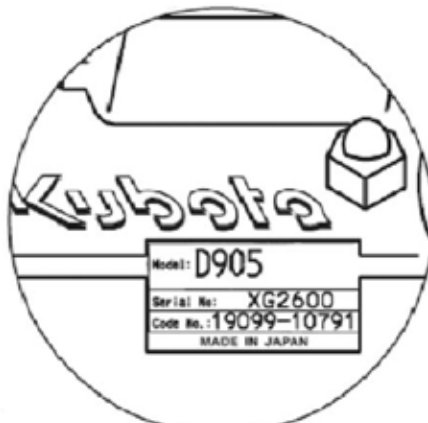
All Models have serial # stickers on the valve cover.
